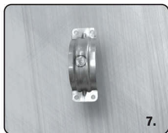
Tailpipe Clamp with Pin Cessna 150 and A150 Replaces: 0450338-9 PN: A0450338-9 PMA New-outright: $19 Can be used for both left and right sides.
