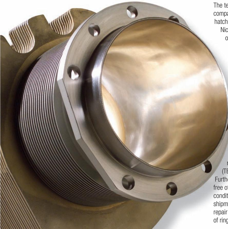
RAM Nickel New or Premium *ValueTime* Overhauled Nickel Cylinders are available for the following engines:
